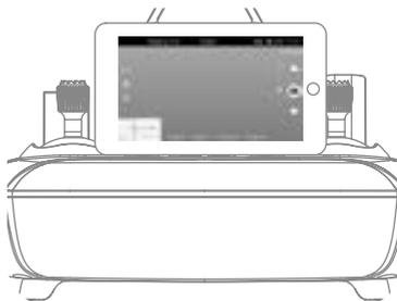
(4) Adjust the phone holder until the phone is fixedly mounted until the phone is fixedly mounted.
